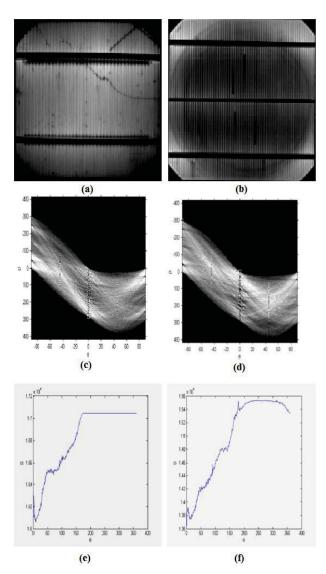
Fig.4. (a) Crack image after cropping, (b) Good image after cropping, (c) Hough transform of Crack image, (d) Hough transform of Good image, (e) S measure of Crack image, (f) S measure of Good image
