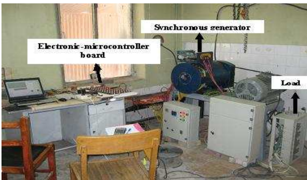
Fig. 5: Testing laboratory and experimental test setup.
