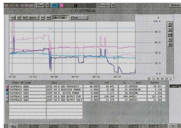
Fig. 2: An actual record of unit #6 of RPC plant during parallel operation with local 132 kV network. Steady oscillation in reactive power output of generator.
