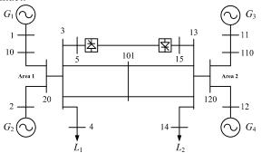
Fig. 3. Two-area test-system with an HVDC-link [12]
