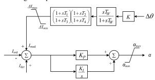
Fig. 4. Transfer function diagram of HVDC supplementary controller
