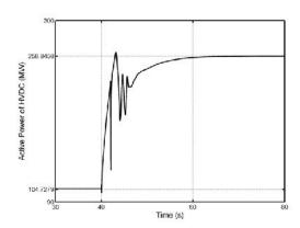
Fig. 15. Active power of DC-link in scenario 2
