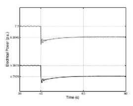
Fig. 12. Electrical power produced by generators in area 1 (solid:  $G_1$ , dashed-dotted:  $G_2$ ), scenario 1
