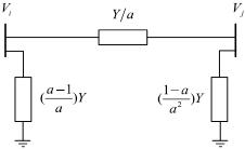
Fig.3. The equivalent- $\pi$  model.
