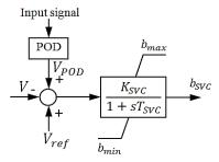
Fig. 4. Block diagram of SVC.
