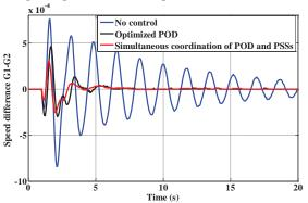
Fig. 18. Speed difference response of G1-G2 for case 2.
