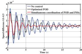
Fig. 17. Speed difference response of G1-G3 for case 1.
