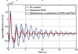
Fig. 16. Speed difference response of G1-G2 for case 1.
