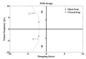
Fig. 12. Open and closed loop eigenvalues (only POD).
