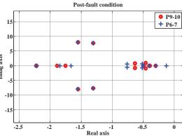
Fig. 11. Zero plots of transfer functions related to SVC output and P<sub>10-9</sub> and P<sub>6-7</sub>.
