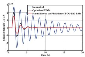
Fig. 19. Speed difference response of G1-G3 for case 2.
