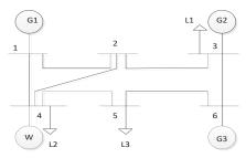
Fig. 5. six-bus system with wind farm
