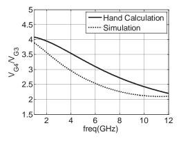
Fig. 19. Hand Calculation and Simulation of Voltage Gain  $V_{\rm G4}/V_{\rm G3}$
