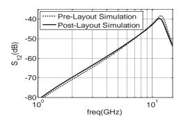
Fig. 25. Simulated reverse gain(dB)
