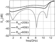
Fig. 12. Effect of variation of RF2 on S11 of the LNA
