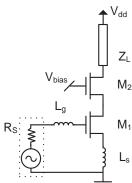
Fig. 2. Narrowband Cascode Source Degenerated LNA Topology
