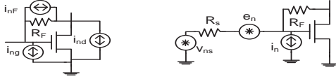
Fig. 8. (a) Three main noise source (b) Classic input referred noise as e_n and i_n
