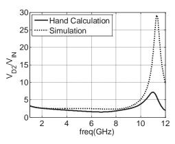
Fig. 21. Hand Calculation and Simulation of Voltage Gain  $V_{\rm D2}/V_{\rm IN}$
