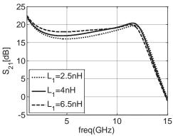
Fig. 13. Effect of variation of L<sub>1</sub> on S<sub>21</sub> of the LNA
