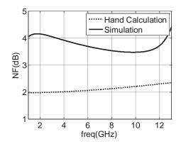
Fig. 22. Hand Calculation and Simulation of Noise Figure
