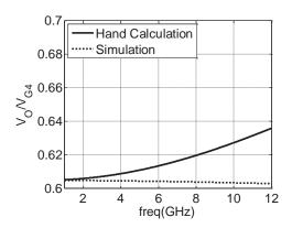
Fig. 18. Hand Calculation and Simulation of Voltage Gain  $V_{\rm O}/V_{\rm G4}$
