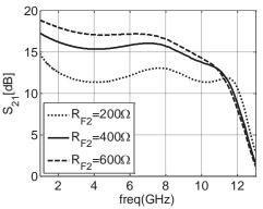
Fig. 17. Effect of variation of R<sub>F2</sub> on S<sub>21</sub> of the LNA
