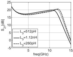
Fig. 15. Effect of variation of L<sub>3</sub> on S<sub>21</sub> of the LNA
