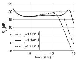
Fig. 14. Effect of variation of L<sub>2</sub> on S<sub>21</sub> of the LNA
