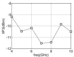
Fig. 30. Simulation IIP3 versus intermodulation frequency
