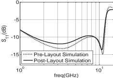
Fig. 26. Simulated input return loss(dB)
