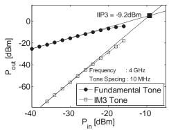
Fig. 29. Simulated IIP3 at 4 GHz
