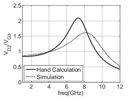
Fig. 20. Hand Calculation and Simulation of Voltage Gain  $V_{\rm G3}/V_{\rm D2}$
