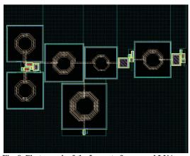
Fig. 9. Photograph of the Layout of proposed LNA
