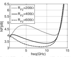
Fig. 11. Effect of variation of R<sub>F2</sub> on NF of the LNA
