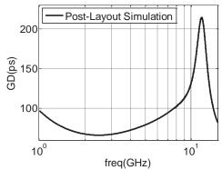
Fig. 28. Simulated Group Delay(ps)
