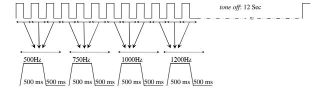
Fig. 14: Illustration of one epoch (block) of the stimulus profile for an auditory excitation. Each epoch contains 12 seconds of *tones on* and 12 second of *tones off* period. During the *tones on* period, 3 tone bursts were presented with a 15 ms rise/fall time at a rate of one per second for each of 4 tone frequencies 500Hz, 750 Hz, 1000 Hz, and 1200 Hz. MEG data of both subjects containe 50 epochs.
