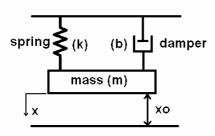
Fig. 3: dynamic mechanical model for MEMS variable capacitor
