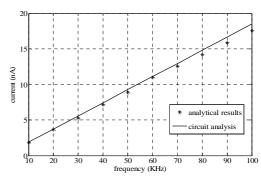
Fig. 7: Capacitor current with 100mV sinusoidal excitation versus frequency (results of analytical calculations and circuit analysis)
