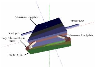
Fig. 1: Schematics of the MEMS variable capacitor
