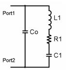
Fig. 5: Equivalent circuit model for small signal analysis
