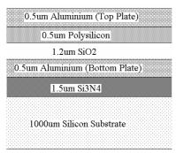
Fig. 2: Profile of The MEMS Layers
