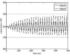
Fig. 6: Capacitance variation versus time with 100-200mV small signal excitation
