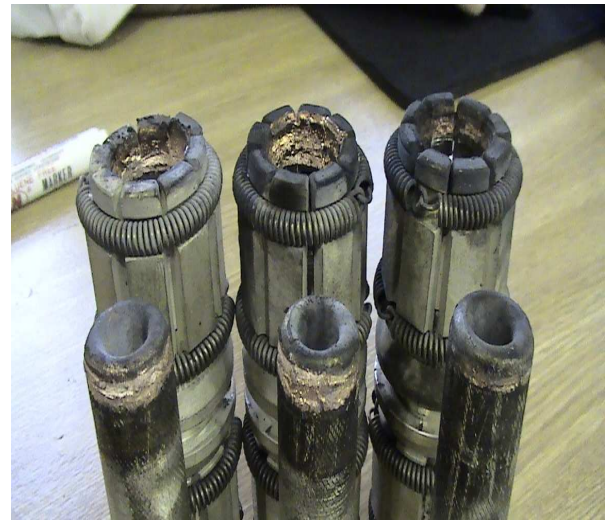
Fig. 8. Failed specimen in CESI laboratory direct tests
