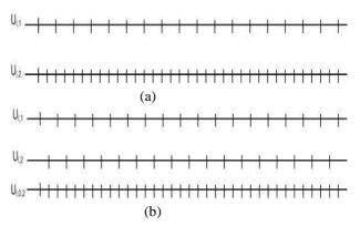
Fig. 4: Quantization schemes and the corresponding signals for: (a) MLC based RDSC system with two encoders, and (b) MDC based RDSC system with two encoders.
