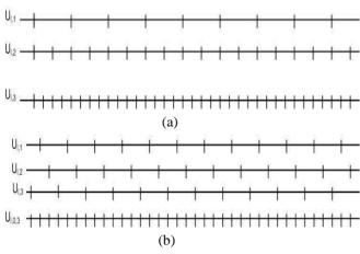
Fig. 5: Quantization schemes and the corresponding signals for: (a) MLC based RDSC system with three encoders, and (b) MDC based RDSC system with three encoders.
