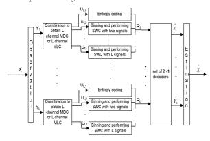
Fig. 3: RDSC using Slepian-Wolf-Cover coded quantization framework
