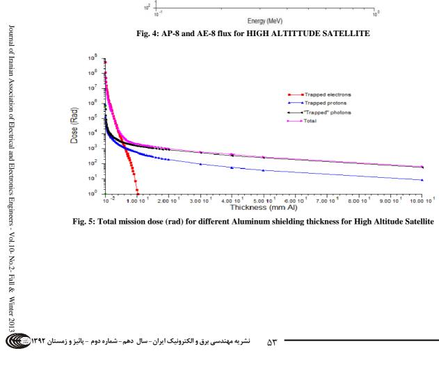
Fig. 5: Total mission dose (rad) for different Aluminum shielding thickness for High Altitude Satellite
