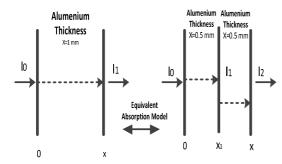
Fig. 2: Absorption thickness base Decomposition process
