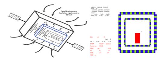
Fig. 7: Reduction steps of radiation for 18-year mission length of HIGH ALTITTUDE SATELLITE
