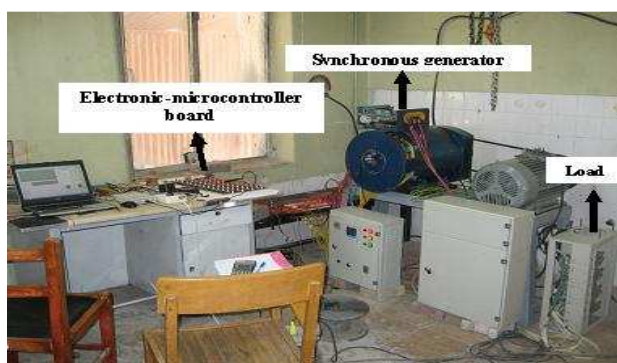
Fig. 5: Testing laboratory and experimental test setup.
