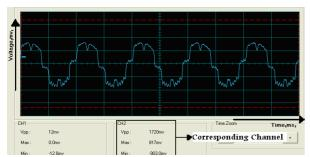
Fig. 9: Measured voltage under healthy operation (no-load).
