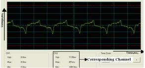
(b) Load level= 7% - Under faulty operation.
