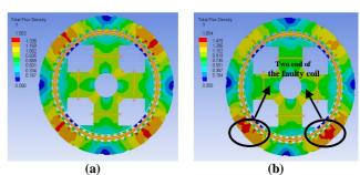
Fig. 4: Distribution of magnetic field density in salient-pole synchronous generator (front view). (a) Under healthy condition. (b) Under turn-to-turn short circuit in stator winding.
