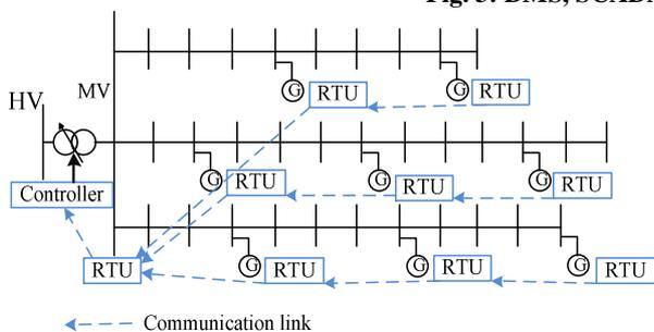
Fig. 4: Structure and position of equipments in proposed approach
