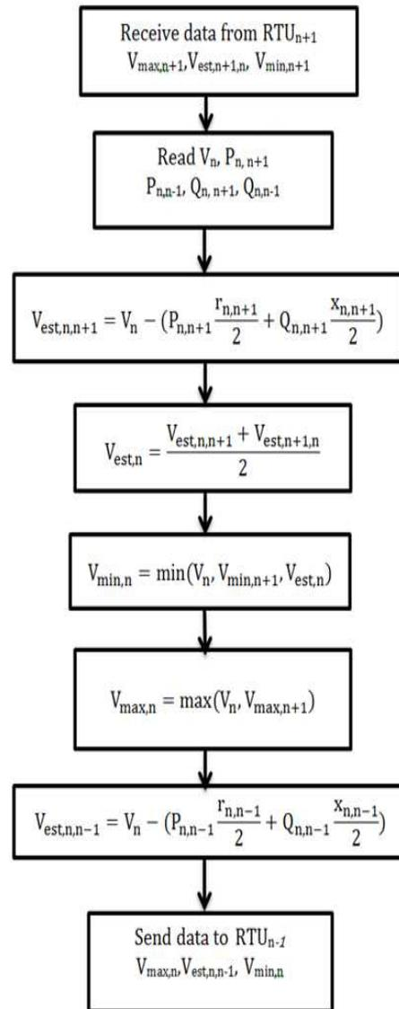
Fig. 6: Procedure of RTU<sub>n</sub>.
