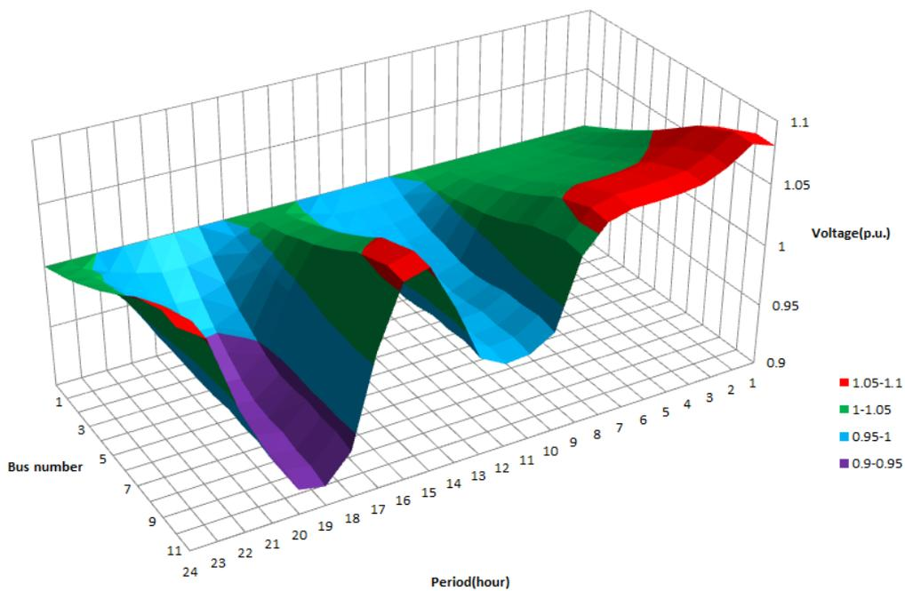
**Fig. 14: Voltage profile of feeder 1 before regulation**
