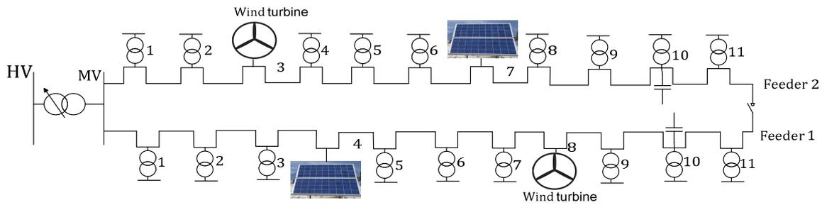
Fig. 7: System used for simulations
