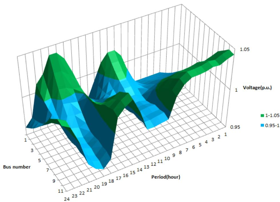
**Fig. 15: Voltage profile of feeder 1 after regulation**
