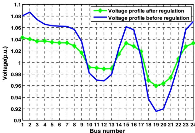
Fig. 18: Voltage profile before and after regulation in bus 11 on feeder 1
