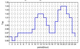
Fig. 13: Tap position based on load flow
