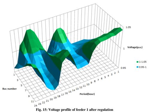
Fig. 15: Voltage profile of feeder 1 after regulation
