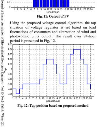
Fig. 12: Tap position based on proposed method
