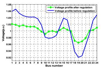
Fig. 19: Voltage profile before and after regulation in bus 11 on feeder 2
