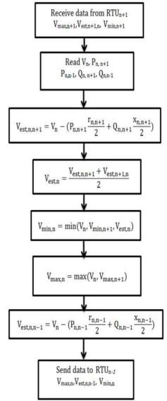
Fig. 6: Procedure of RTU<sub>n</sub>.
