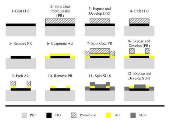
Fig. 1. Process flow of ITO/PET microelectrode Array fabrication.
