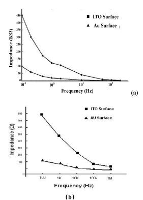
Fig. 7. Impedance characteristics of ITO and gold stimulation sites, (a) 7854µm² contact area, (b). 3mm² contact area.
