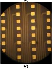
Fig. 3. (a) Fabricated biomimetic microelectrode array with 72 sites 100-μm-diameter electrodes with ITO on PET substrate (b, c) stimulation sites of visual prosthesis electrode array covered with gold. circular
