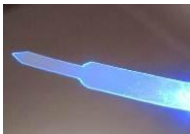
Fig. 8. Prepared electrode for surgical implantation
