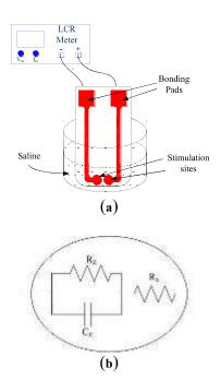
Fig. 6 (a) Impedance test diagram, (b) equivalent circuit
