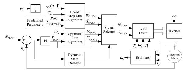
Fig. 9. Block diagram of proposed speed drop minimization algorithm
