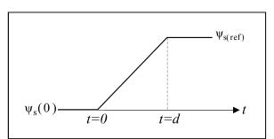
Fig. 6. The proposed reference flux.
