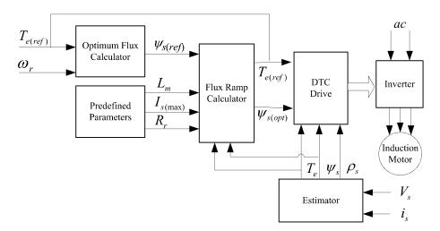
Fig. 7. Block diagram of proposed current limiting algorithm
