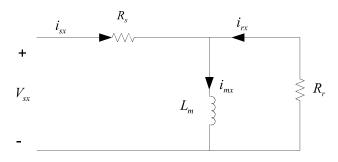
Fig. 4. Simplified x-axis equivalent circuit
