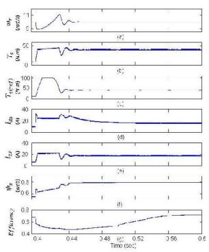
Fig. 13. DTC-SVM drive with the speed controller using speed drop minimization algorithm (a)Speed, (b) Electrical torque, (c) Torque reference, (d-e) d and q axis components of stator current in stator flux reference frame, (f) Stator flux, and (g) Efficiency of motor.
