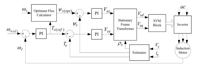
Fig. 1. Block diagram of DTC-SVM and loss minimization
