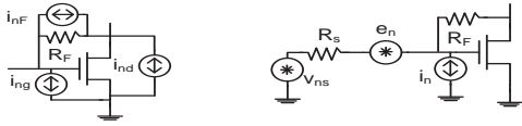
Fig. 8. (a) Three main noise source (b) Classic input referred noise as e_n and i_n
